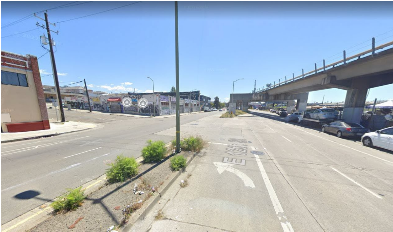
H-6 | E12 th Street at 19 th Avenue in Oakland: Lack of marked pedestrian crossings for long stretches of E12 th Street leads to jaywalking and unsafe conditions
