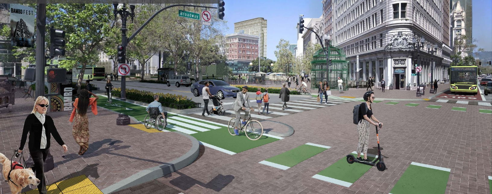
Planned Improvements at 14th St and Broadway, including protected bike lanes, directional curb ramps, etc
